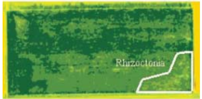
IKONOS derived NDVI for selection of beet acres for destruction under PIK program
